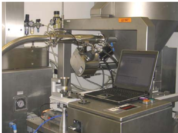
Figure 7: Very narrow conditions for a \varnothing 50 mm sampler TWISTER and GMP-Module; analyser within a mobile rack
