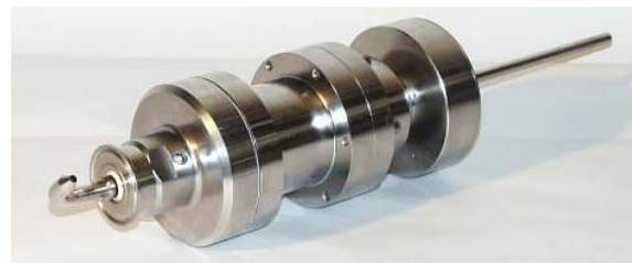
Figure 2: Pivoting L-probe as an example for non-representative sampling.
