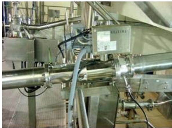
Figure 8: Sampler in 150mm horizontal product line.
