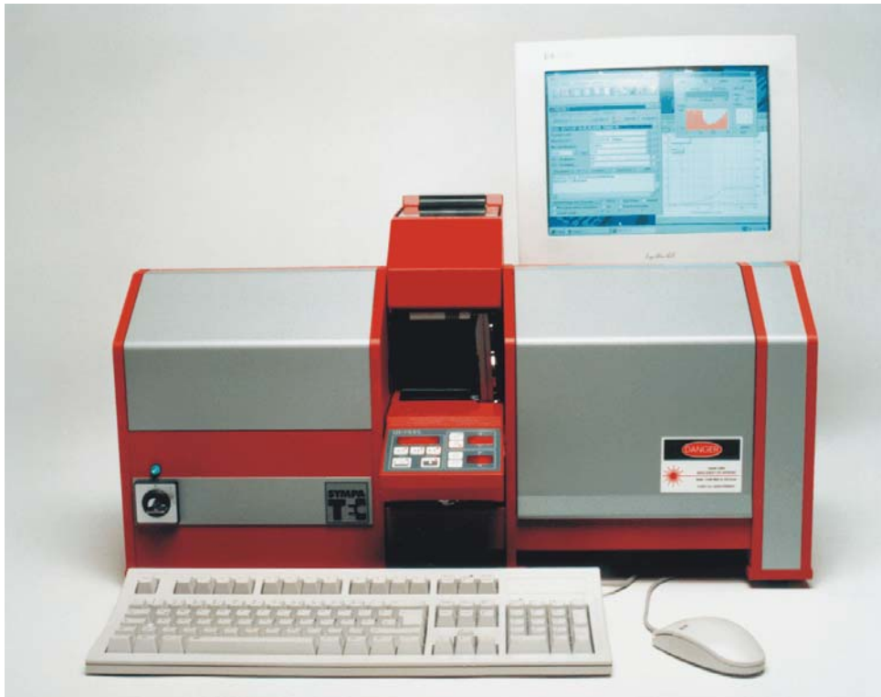
Fig. 8 Current off-line technology (i.e. lab-applications) for wet dispersion (Sympatec HELOS/BF with QUIXEL)
