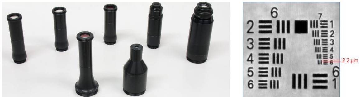
Fig. 4: Measuring ranges M3 and M9 (left, front) and USAF resolution target imaged by M3 (right)
