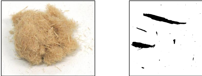
Fig. 8: Sample of wood fibres and a typical image created by QICPIC with measuring range M9
