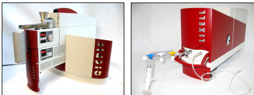
Figure 1: (left) OASIS, comprising the wet (SUCELL, top) and dry disperser (RODOS, bottom) inserted into the measuring zone of the HDIA system QICPIC; (right) wet disperser LIXELL with syringe and valves connected.
