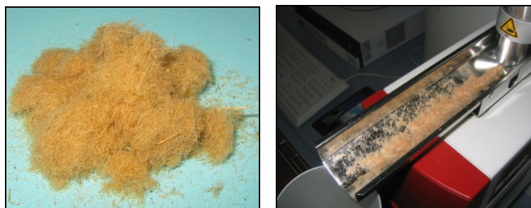
Figure 6: Original wood fibres (left), manually pre-dispersed fibres in the chute of a vibratory feeder VIBRI (right) feeding to the funnel of the dry disperser RODOS/L.
