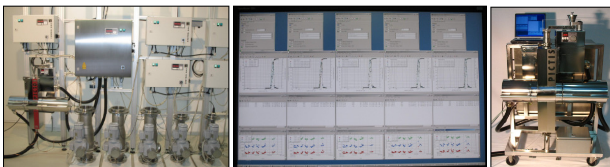
Figure 4: (left) PICTOS combined with five TWISTER, (centre) process control of five pipes in the polystyrene production, (right) PICTIS with built-in gravity disperser, mounted on a trolley for GMP applications.
