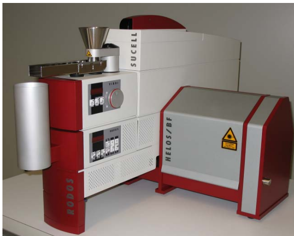
Figure 2: OASIS/L wet and dry dispersing system set-up in the HELOS laser diffraction sensor.
