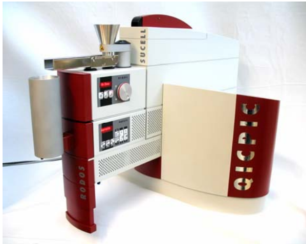
Figure 1: OASIS/L wet and dry dispersing system set-up in the QICPIC image analysis sensor.
