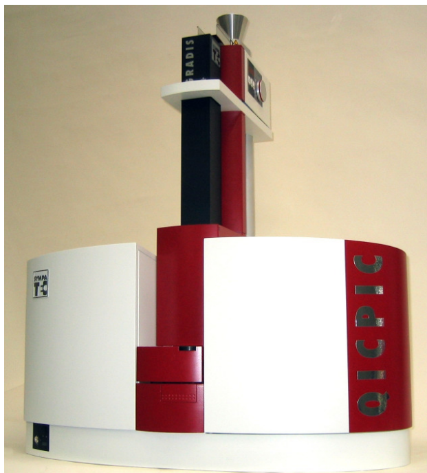
Figure 5: Set-up of the DIA system QICPIC™ with gravity disperser GRADIS/L™ and dry feeder VIBRI/L™
